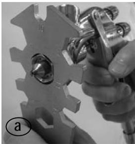
a. Disassembly fluid nozzle (2-1),
