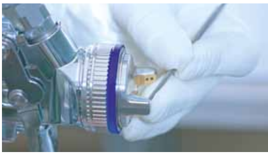
Manual adjustment: Each nozzle set is manually "tuned" in order to ensure an optimum spray pattern.
